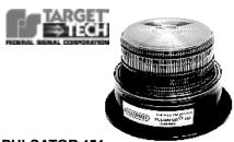
PULSATOR 451 8 joule power supply, 12 to 48VDC. Applications: Snowplows, highway vehicles. Double flash. Enclosed polycarbonate base. 4" tall, 6-1/2" diameter. Amber: Part No. 211680-02 Clear: Part No. 211680-05 Heavy Duty Version: (Gel-filled base-protection) Amber: Part No. 211823-02
